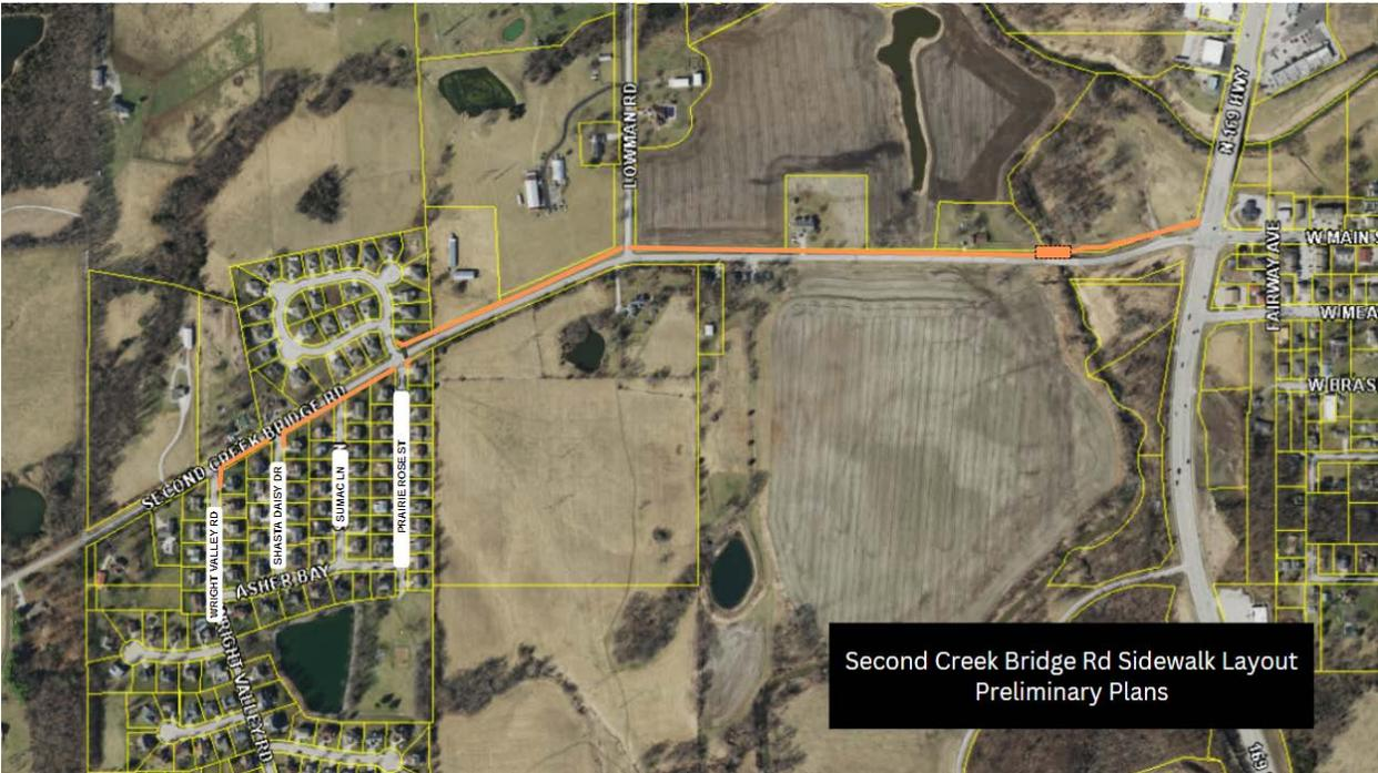
The Riverwalk Trail will feature an 8-foot-wide concrete sidewalk extending from Heritage Park to Highway 169, where it will connect to the Second Creek Bridge Road Sidewalk Project. The trailhead will begin at the parking lot on the east side of Heritage Park, cross US 169 beneath the bridge, and continue to connect with Second Creek Bridge Road.
